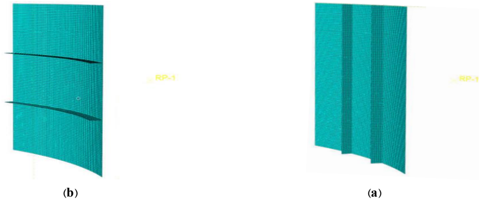
Fig. 3. Geometry the model of FGM cylindrical shells with longitudinal (a) and circular (b) stiffeners
