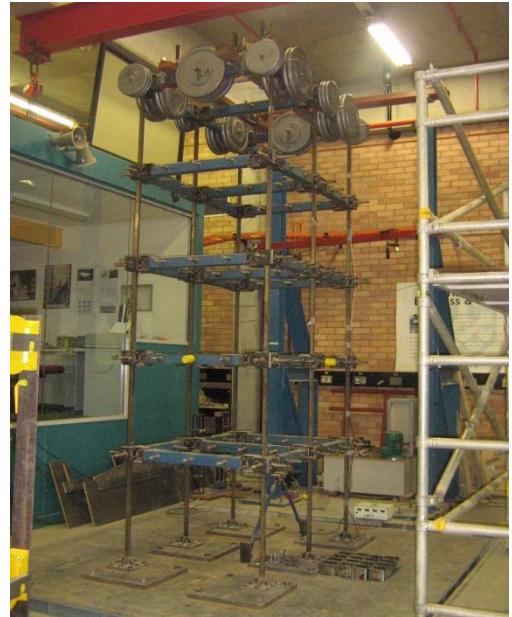
Fig. 2. The 5-story benchmark structure [3].
