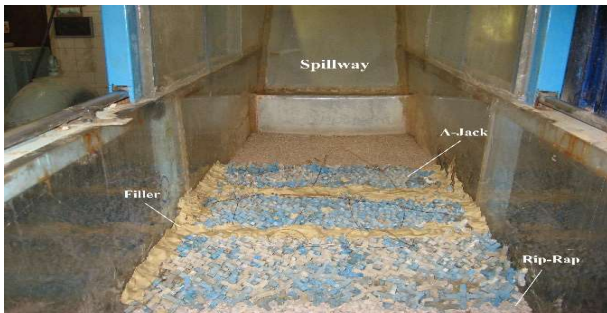
Fig 1. The protected bed with SLC and rip-rap materials
