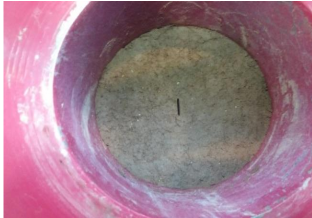
Fig. 3. Crack created in samples
