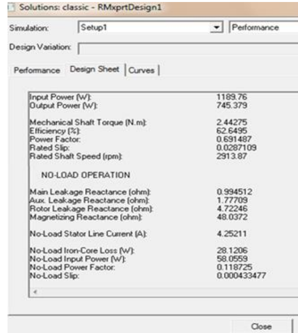
Fig.14. Results of FEM analysis for the motor designed by conventional method
