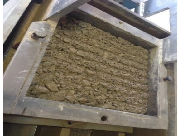
Fig. 2. Preparation of the filter materials at the lower half of the direct shear box
