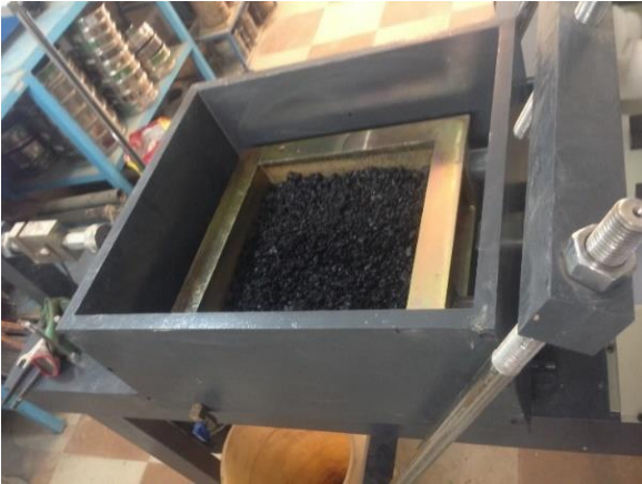
Fig. 1. Preparation of the asphalt mix at the lower half of the direct shear box
