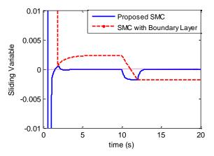
Fig. 14. Sliding Variable using Proposed SMC and Boundary Layer SMC (Sliding Phase).
