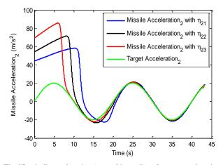
Fig. 27. missile acceleration (control input 2) and target acceleration (uncertainty) with  $\eta_{21} < \eta_{22} < \eta_{23}$ .
