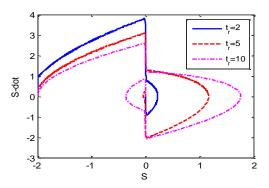
Fig. 19. Reaching Phase using Proposed SMC with  $t_r = 2,5,10$ .
