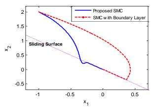
Fig. 17. System Trajectory using Proposed SMC and Boundary Layer SMC in the Phase Plane.
