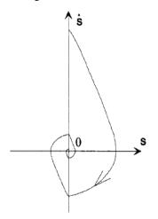
Fig. 5. Twisting controller trajectory in the phase plane
