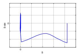
Fig. 1. 1-SMC reaching phase (Sliding takes place on the S = 0 axis)
