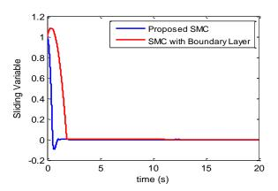
Fig. 13. Sliding Variable using Proposed SMC and Boundary Layer SMC.
