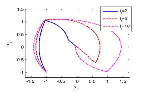
Fig. 21. System Trajectory using Proposed SMC with  $t_r = 2,5,10$ in the Phase Plane.
