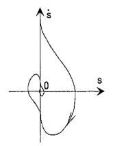
Fig. 6. Super Twisting controller trajectory in the phase plane
