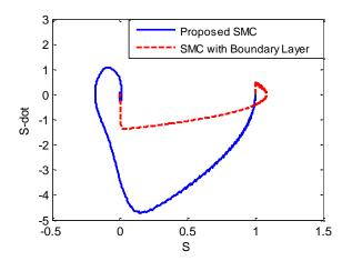
Fig. 12. Reaching Phase using Proposed SMC and Boundary Layer SMC.
