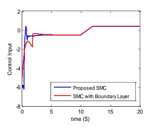
Fig. 11. Control Input Signal using Proposed SMC and Boundary Layer SMC.
