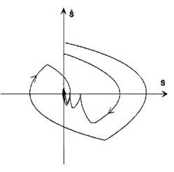
Fig. 4. The two possible trajectories of the sub-optimal algorithm in the phase plane
