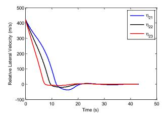
Fig. 28. relative lateral velocity (sliding variable 2) with different value for  $\eta_2$  ( $\eta_{21} < \eta_{22} < \eta_{23}$ ).
