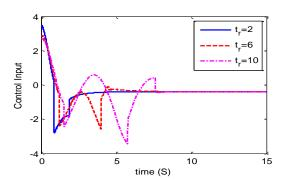
Fig. 18. Control Input Signal using Proposed SMC with  $t_r = 2,5,10$ .
