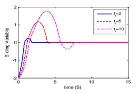
Fig. 20. Sliding Variable using Proposed SMC with  $t_r = 2,5,10$ .
