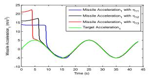
Fig. 23. missile acceleration (control input 1) and target acceleration (uncertainty) with  $\eta_{11} < \eta_{12} < \eta_{13}$ .
