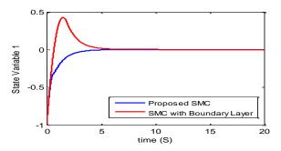
Fig. 15. State Variable 1 using Proposed SMC and Boundary Layer SMC.
