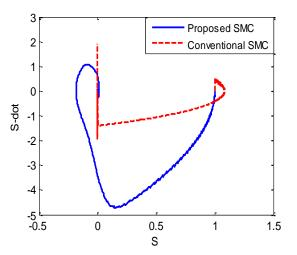
Fig. 10. Reaching Phase using Proposed SMC and Conventional SMC.
