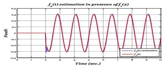
Fig. 5. The  $f_2(t)$  estimation with effect of  $f_1(t)$
