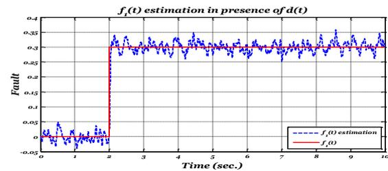
Fig. 6. The  $f_1(t)$  estimation with effect of  $d(t)$
