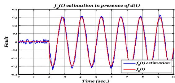
Fig. 7. The  $f_2(t)$  estimation with effect of  $d(t)$
