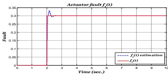
Fig. 2. The  $f_1(t)$  and its estimation
