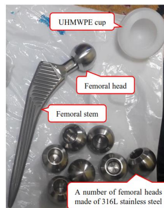
Fig. 3. Actual view of some samples of metal femoral heads with an artificial hip joint.
