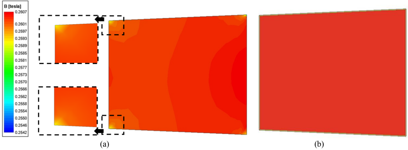
Fig. 13. Demagnetization analysis results of ferrite PM (a) No-load (zero torque transmission position) magnetic field distributions (b) Full-load (maximum torque transmission position) magnetic field distribution
