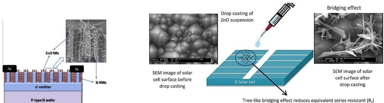
**Fig. 8.** schematic of the proposed Si nano-textured solar cell. The inset is the SEM image of ZnO NRs.
