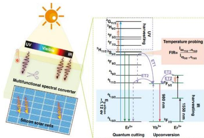
Fig. 12. A schematic illustration of multifunctional  $\text{NaY}(\text{WO}_4)_2: \text{Er}^{3+}/\text{Yb}^{3+}$  phosphors mounted on the front of silicon solar cells to enhance their performance.
