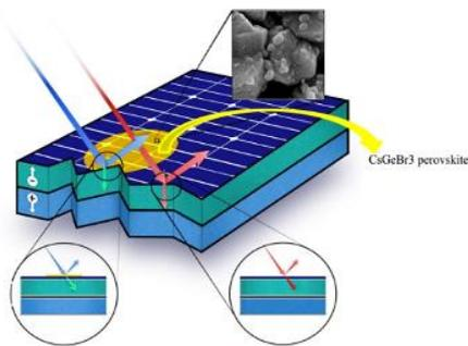
**Fig. 10.** Drop-casting schematic of the CsGeBr<sub>3</sub> suspension on the Silicon solar cell and SEM image of the CsGeBr<sub>3</sub> perovskite powder.
