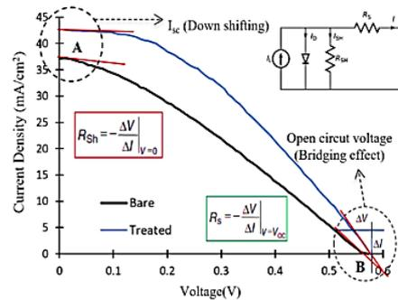
Fig. 2. Typical I-V characteristics of Si solar cell;  $R_s$  and  $R_{sh}$  for untreated and treated solar cell.
