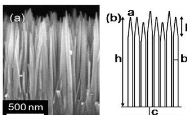
**Fig. 6.** Example of ZnO NR, Cross section SSEM image of a highly tapered ZnO NRA.
