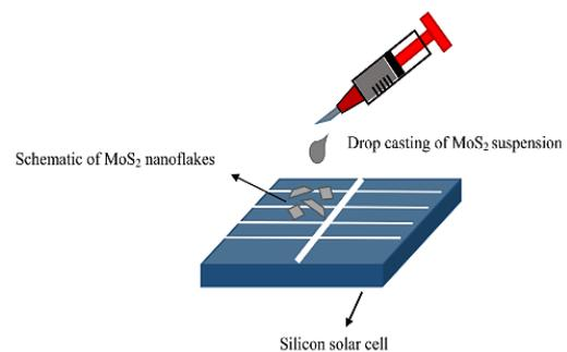
**Fig. 11.** Drop-casting schematic of MoS<sub>2</sub> suspension.
