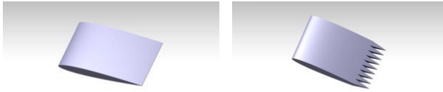
Fig. 1. Geometry of the NACA 0012 airfoil. Left) baseline model, right) serration model.
