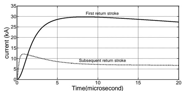
**Fig.1. Channel-base current waveshapes for typical first and subsequent return strokes**
