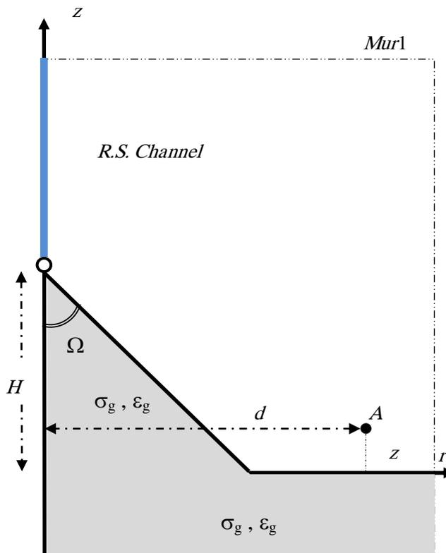
Fig. 2. Lightning strikes to a cone-shaped ground in two dimension view
