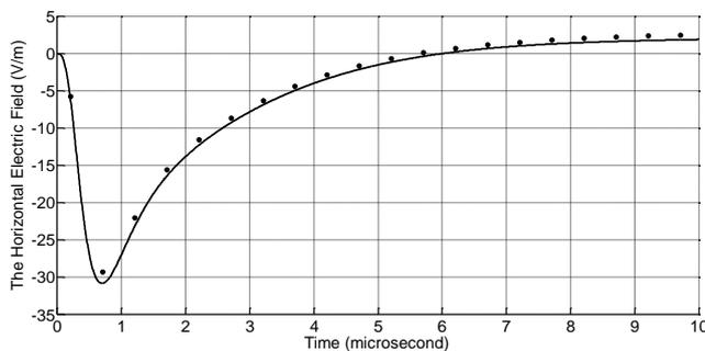
**Fig. B1. The determined horizontal electric field using cylindrical 2D-FDTD method (solid line) and Equ. (B1) (dot marker)**
