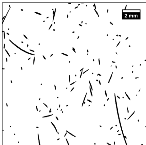
Fig. 1. A processed image of the cross-section of the copper fiber/resin composite using ImageJ software.
