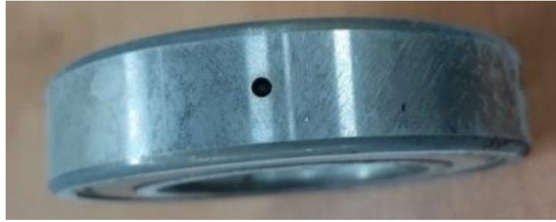
Fig. 2. The hole created in the outer ring of the bearing to speed up the run-to-failure test (highly accelerated life test: HALT)
