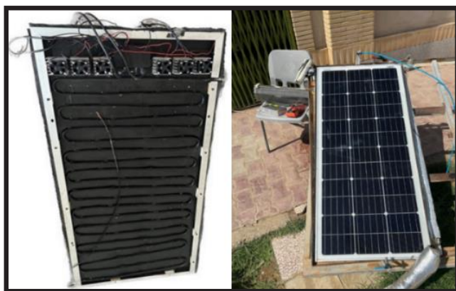
Fig. 1. Photovoltaic/thermal laboratory system with thermoelectric generators, heat sink, and fan.
