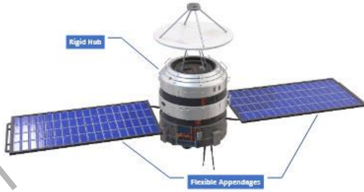
Fig.1.Flexible satellite structure model
