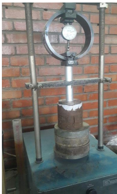
Fig. 10. Procedure for conducting uniaxial compressive strength tests on the studied samples.
