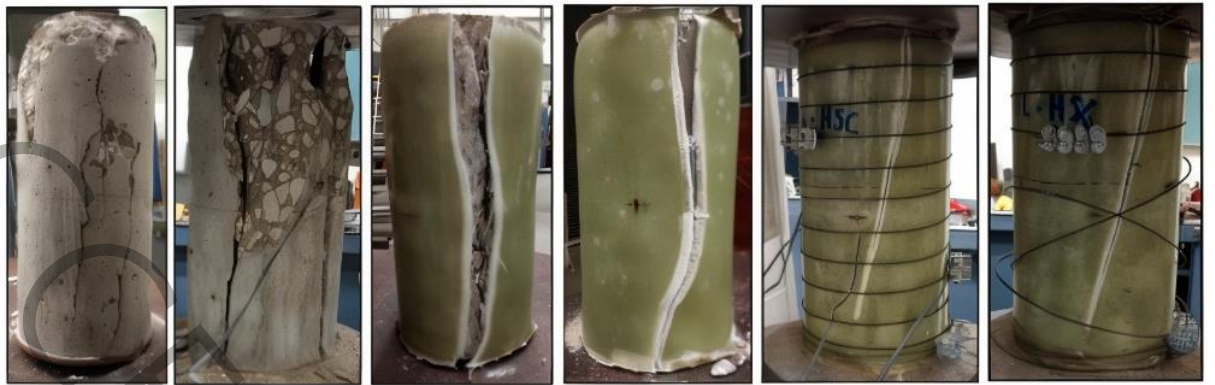
a) Unconfined NSC b) Unconfined HSC c) NSC wrapped with FRP d) HSC wrapped with FRP e) Hybrid confined – at FRP rupture f) Hybrid confined – at SMA rupture
