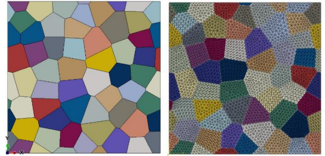
Fig. 2. A sample of Voronoi tessellation and its meshing..
