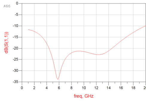
Fig. 4 .Reflection coefficient value of proposed antenna using ADS tool
