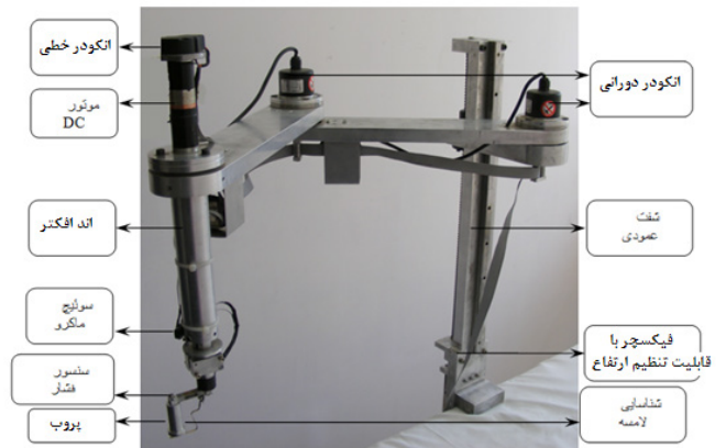
Fig. 1. Design of a tactile sensing robot called "Robotic Tactile Breast Mass Identifier (Robo-Tac-BMI)"
