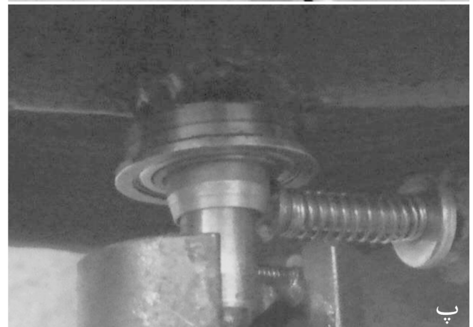
Fig. 5. a) Frontal view of small wind turbine. b) Electrical and mechanical components of wind turbine. c) Installation of mechanical brake and magnet
