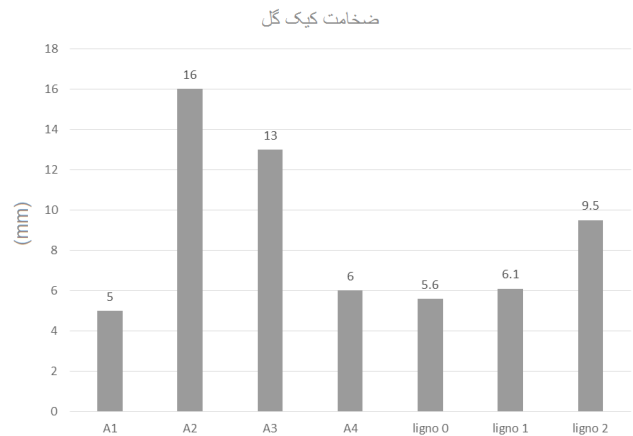
Fig. 5. Measured thickness of mud cakes
