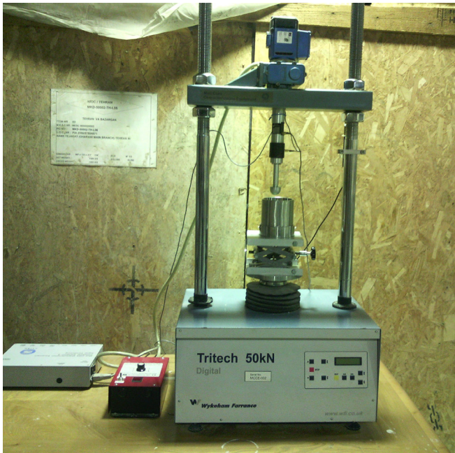
Fig. 3. Mud Cake Characterization Equipment (MCCE)
