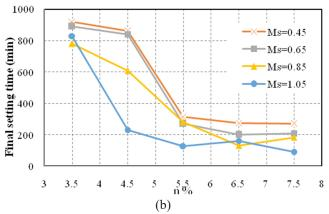
Fig. 3. The effect of alkali solution parameters on setting time of AAS paste: (a) initial setting time and (b) final setting time.
