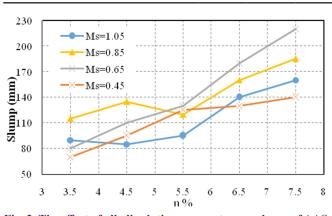
Fig. 2. The effect of alkali solution parameters on slump of AAS concrete.
