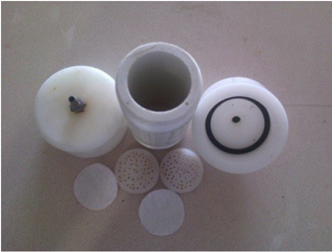
Fig. 3. Typical mold used for sample preparation
