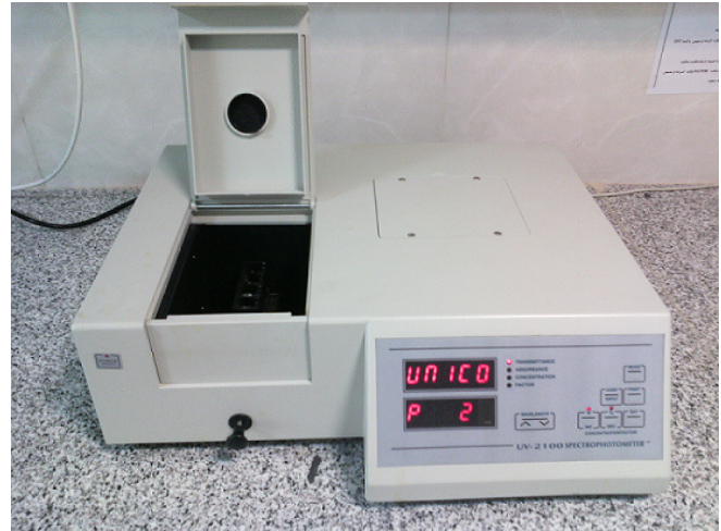
Fig. 2. Spectrophotometer used to indicate concentration of bacterial cell
