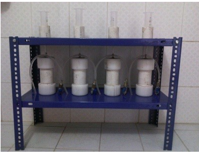
Fig. 4. Set up for gravitational injection at controlled rate
