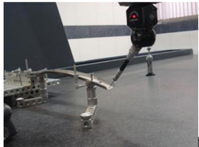
Fig. 7. Experimental sample measurement by CMM
