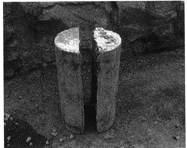
Figure 9a: Failure Mode of concrete after splitting tensile loading.
