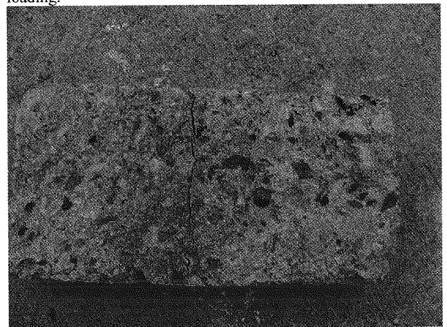
Figure 9b: Rubber particles distribution in concrete matrix after failure on tensile loading.
