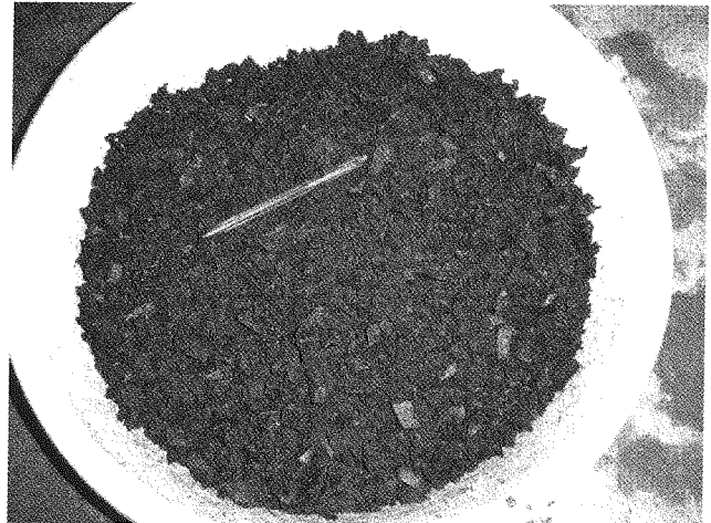
Figure 3: Rubber shredded (Chip rubber particles) as replacement for coarse aggregates.
