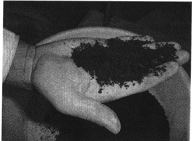
Figure 4. Rubber powder as replacement for cement.
