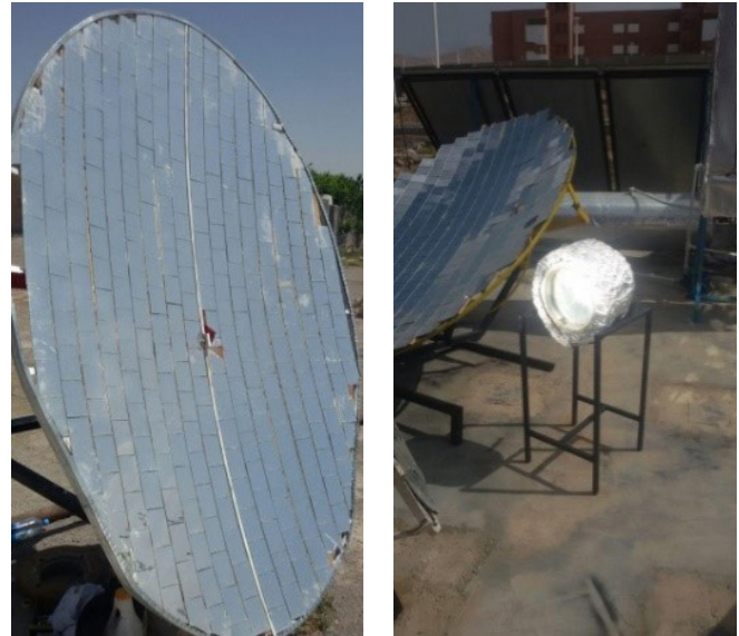
Fig. 12. A view of the manufactured Scheffler concentrator with its receiver
