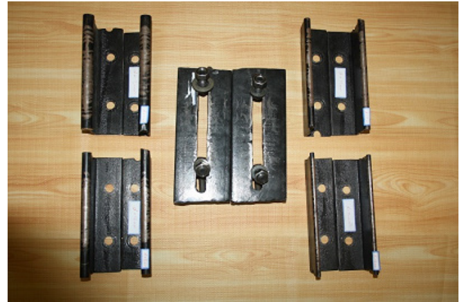
Fig.1. The Set of adjustable-distance cylindrical indenters with diameter of 8, 12, 16 and 20 mm.
