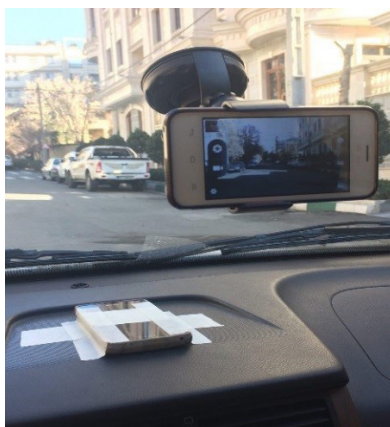
Fig. 3. Smartphones attached over the dashboard and on the car windshield
