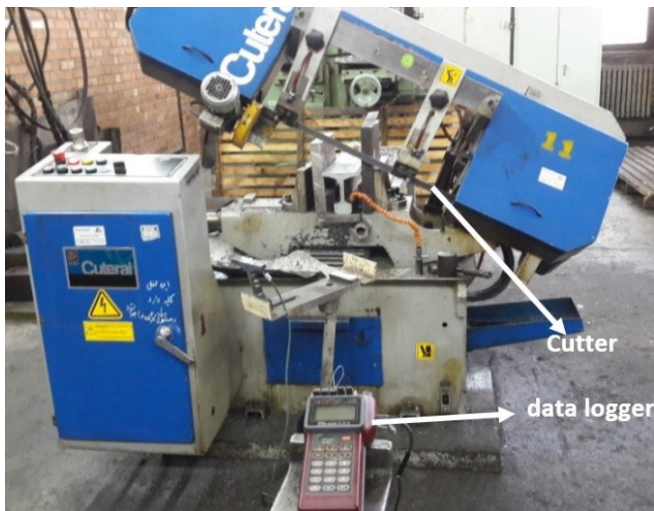
Fig. 14. The used equipment in sectioning test
