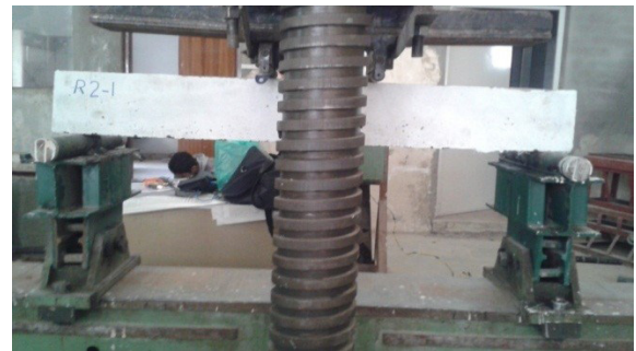
Figure 3. One of the beams under testing
