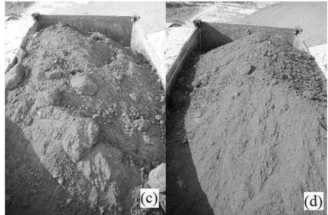
Fig. 3. Accumulation of materials on (a) rear, (b) uniform, (c) right and (d) left sides of the dump body
