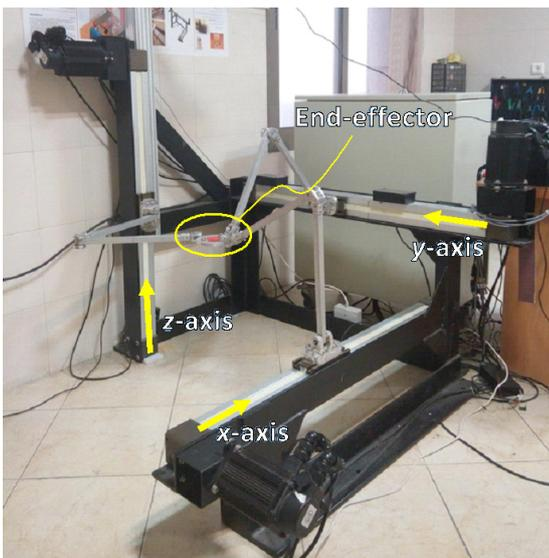
Fig. 1. The 3-DOF decoupled PM constructed in the Human and Robot Interaction Laboratory, University of Tehran.
