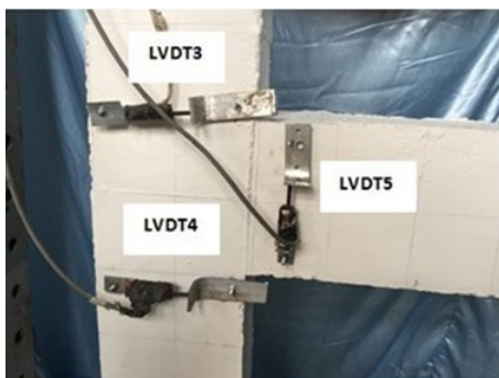
Figure 9. The details of the LVDTs at the connection
