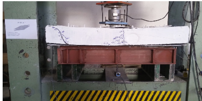
(a) loading and development of cracks in SCSB10-3 slab
