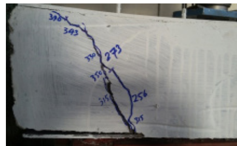
(c) shear crack of concrete and separation of lower plate from concrete
