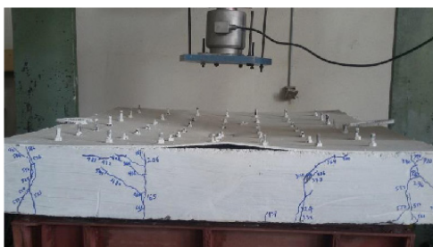
(c) Cracks development in SCSB12-3 sample
