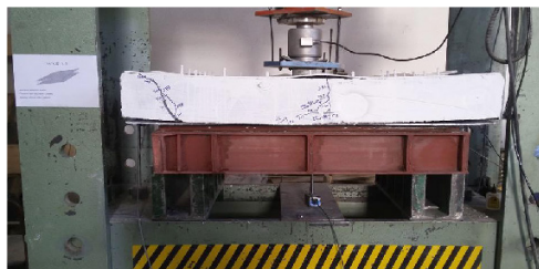
(b) Cracks development in SCSB10-3 sample
