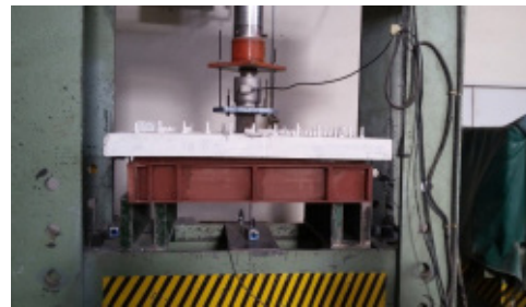
(b) Putting the sample on the support and loading by a rigid component
