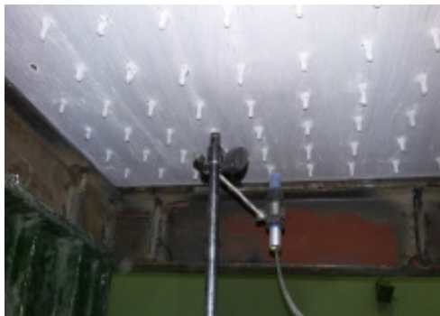
(c) Installation of LVDT in the central point under the sample
