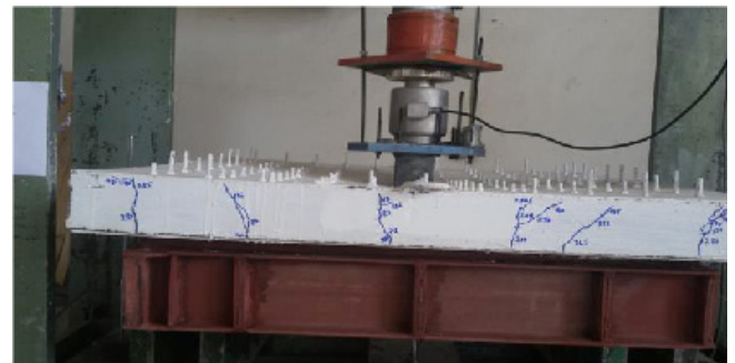
(b) Cracks development in SCSB8-2 sample
