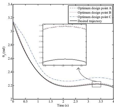
Fig. 5. Tracking trajectory  $\theta_3$  for the optimum design points A, B, and C shown in the Pareto front
