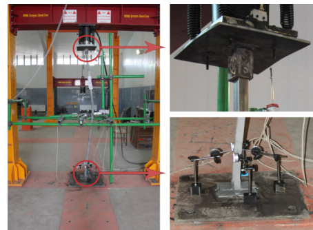
Figure 11. Details of fixed supports in specimens
