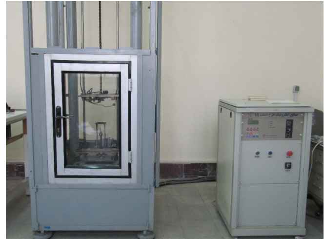
Fig. 3. The Amirkabir Thermo-elasticity Center of Excellence drop hammer test system
