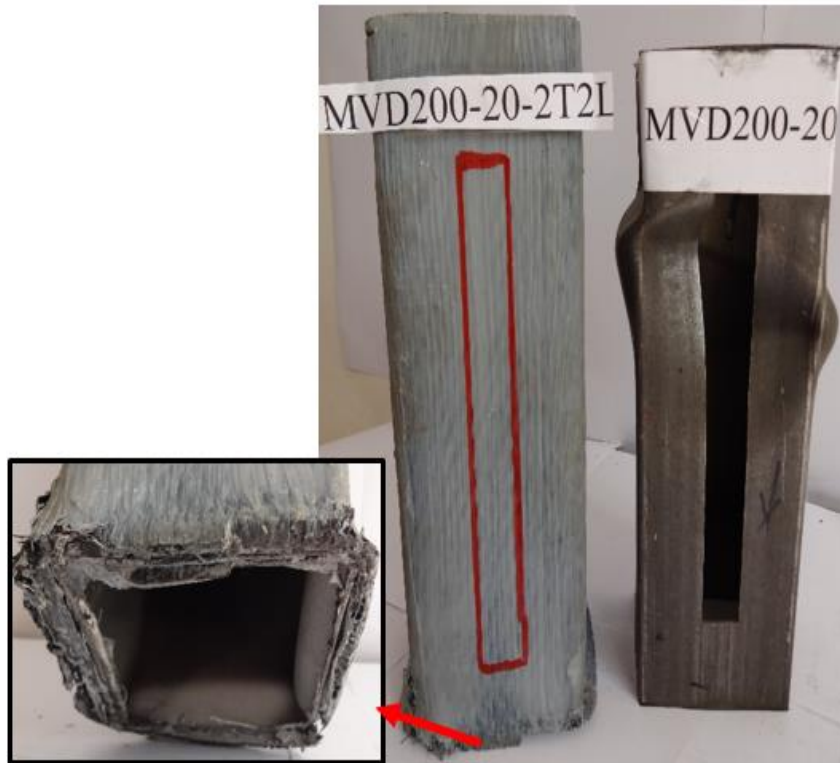
Fig. 9. Failure modes of the specimens with middle deficiency: non-strengthened and strengthened
