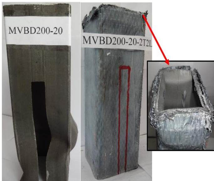
Fig. 10. Failure modes of the specimens with middle-bottom deficiency: non-strengthened and strengthened
