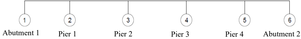
Fig. 3. Layout of stations on the ground compatible with bridge abutment and piers to simulate time histories
