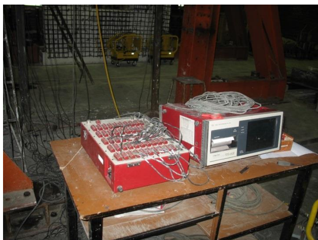
Fig. 9. Data acquisition apparatus (TML)
