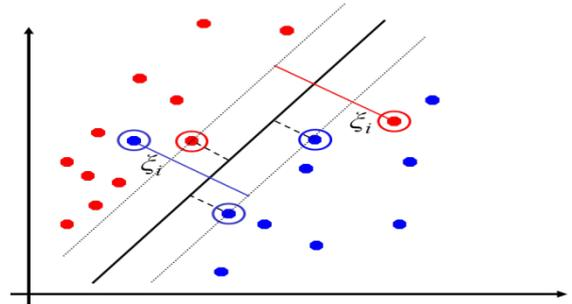
Fig. 5. SVM classification in case of samples which are not linearly separable
