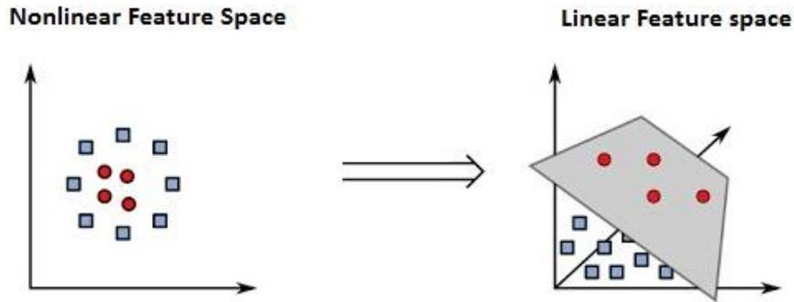
Fig. 6. Nonlinear input space mapped with a kernel function to a linear feature space
