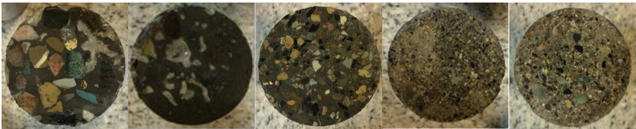
Fig. 1. The cross section of concrete samples made of continuous (the maximum aggregate size of 12.5 mm) and discontinuous aggregate gradation right to left: 1.1-12.5, 1.18-2.38, 2.38-4.75, 4.75-9.5, 9.5-12.5mm.
