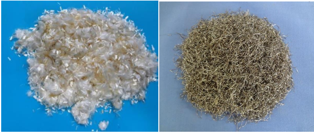
a) b) Fig 1. Used Fibers a) PVA Fiber; b) micro Steel Fiber
