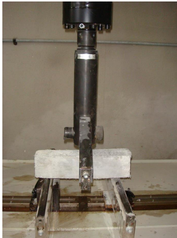
Fig 3. Method of the three-point flexural strength test
