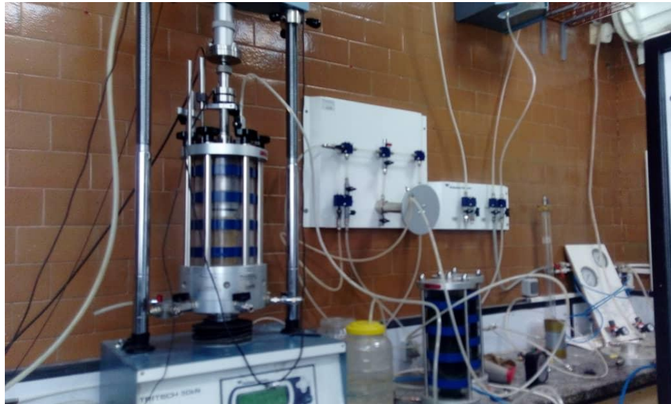
Fig. 13. Undrained cyclic triaxial testing and equipment
