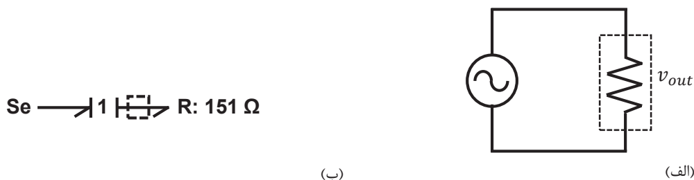
Fig. 7: Embryo model of band pass filter [23]: a) Electrical circuit, b) Bond graph presentation
