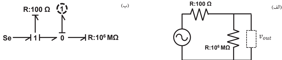
Fig. 14. Embryo model of band stop filter [23]: a) Electrical circuit, b) bond graph presentation
