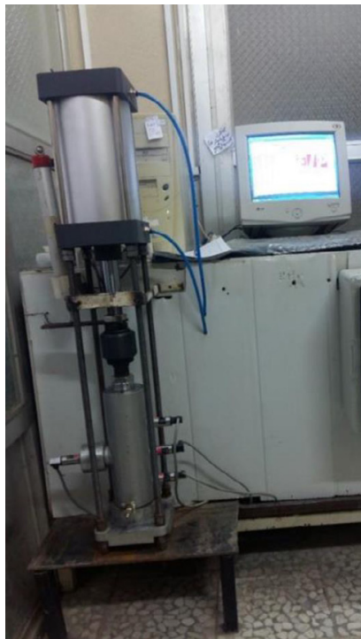
Fig. 8. Tall pneumatic oedometer apparatus
