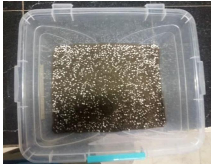
Fig. 6. Sand-EPS beads mixture
