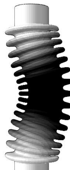
Fig. 2. Bellows column buckling
